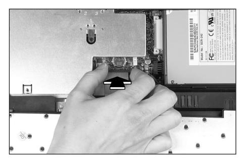
**3** Rotate the keyboard toward the LCD panel until the keyboard is almost face-up.
